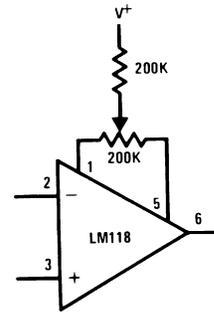
**Figure 39. Offset Balancing**
