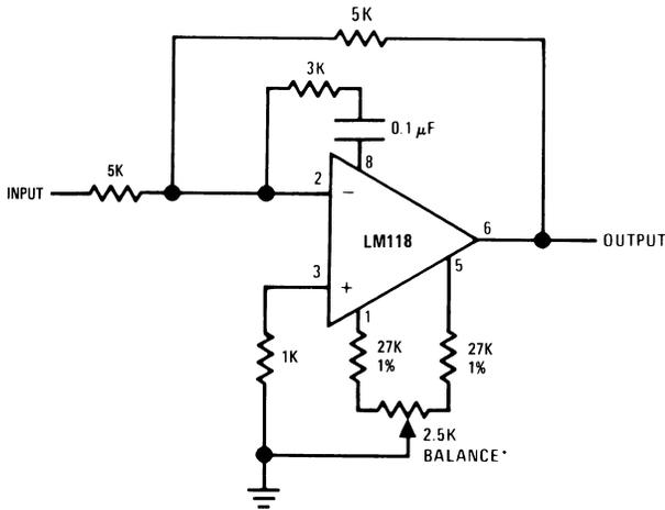
\*Balance circuit necessary for increased slew.
