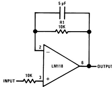
Do not hard-wire as voltage follower ( $R_1 \geq 5 \text{ k}\Omega$ )
