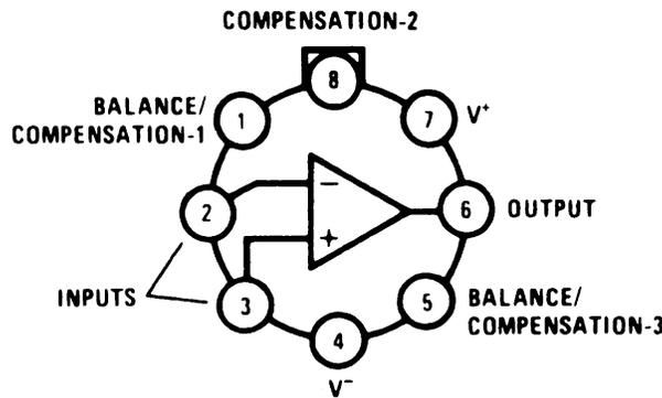
Pin connections shown on schematic diagram and typical applications are for TO-99 package.
