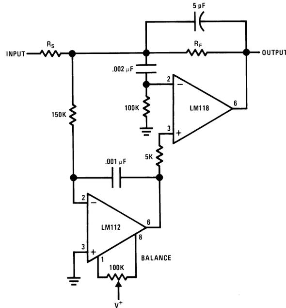
Figure 50. Fast Summing Amplifier with Low Input Current
