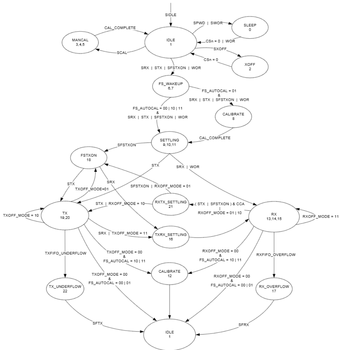
Figure 16: Complete Radio Control State Diagram
