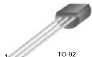
1. Emitter 2. Base 3. Collector
