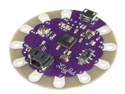
This board operates at 3.3V and features a JST socket to directly connect a Li-Po battery for power. An on-board power switch allows you to turn it off. These boards were designed to streamline sewable projects by keeping things simple. You get more room to work while eliminating the need to sew a power supply. The LiPo battery is even rechargeable through the board, no more special external LiPo chargers required.
