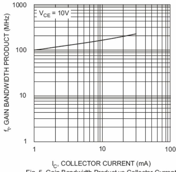
Fig. 5, Gain Bandwidth Product vs Collector Current
