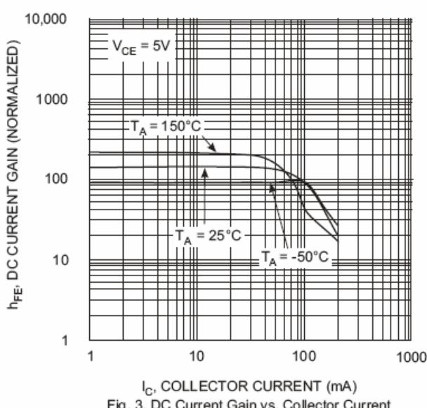
Fig. 3, DC Current Gain vs. Collector Current
