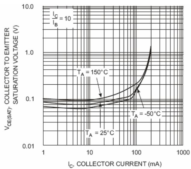
Fig. 2, Collector Emitter Saturation Voltage
