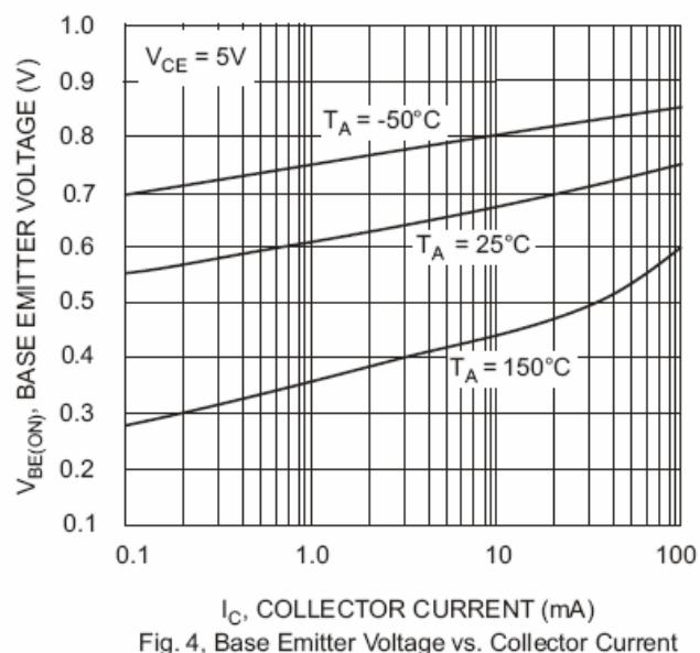
Fig. 4, Base Emitter Voltage vs. Collector Current
