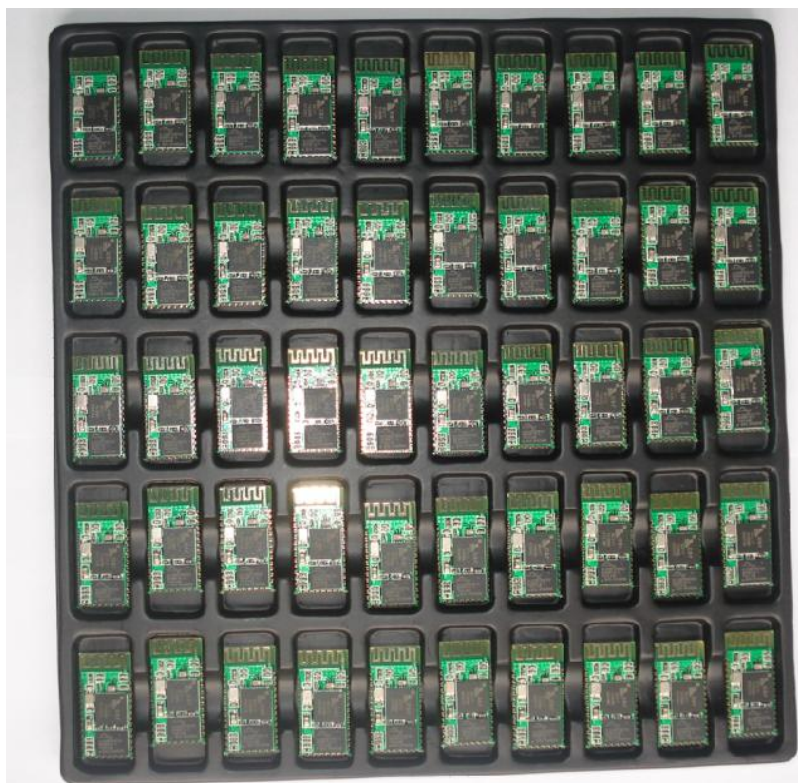
Figure 3 50 pieces chips in an anti-static blister package.
